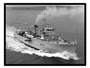
HMS BRONINGTON is one of around 120 Ton-class minesweepers built in the 1950s. With hulls of mahogany, the TONs were the last wooden warships built for the Royal Navy before it switched to today's plastic-hulled Mine Hunters (HUNTs and SANDOWNs) in the 1970s. (More ship details, <u>here</u>).
